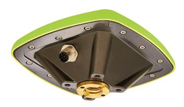
TyrAnt receiver (smart antenna) is based on our TRIUMPH Technology implemented in our TRI-UMPH Chip. The high performance GNSS antenna is integrated together with the receiver in the compact and robust housing. TyrAnt can be mounted on flat surfaces with four screws or mounted on standard poles (5/8-11 or 1-14 inches thread).
