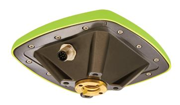
MCAnt-3S receiver is based on our technology implemented in our TRIUMPH3 Chip. 874 GNSS channels of this receiver allow tracking all current and future satellite signals. The high-performance GNSS antenna is integrated together with the receiver in a compact and robust housing. MCAnt-3S can be mounted on flat surfaces with four screws or mounted on standard poles (5/8-11 or 1-14 inches thread).
