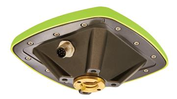
AgAnt-3S receiver is based on our technology implemented in our TRIUMPH3 Chip. 874 GNSS channels of this receiver allow tracking all current and future satellite signals. The high-performance GNSS antenna is integrated together with the receiver in a compact and robust housing. AgAnt-3S can be mounted on flat surfaces with four screws or mounted on standard poles (5/8-11 or 1-14 inches thread).
