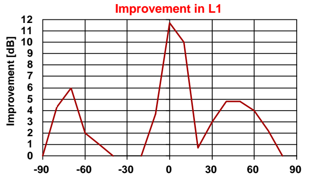
Figure 6. The difference between two ground planes behavior for L1 signal
