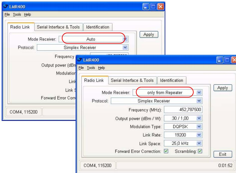
**Figure 2-15. Radio Link tab settings**
