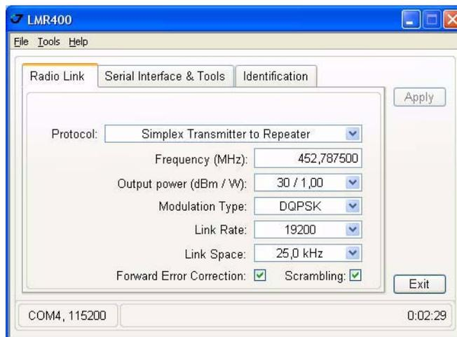
**Figure 2-5. Radio Link tab settings**
