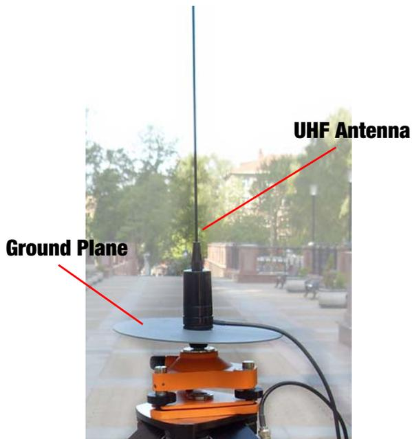
Use coaxial cable and connectors that are impedance-matched with the radio equipment, and make sure to use the shortest length of cable to move the signal between the radio and the antenna, e.g.
