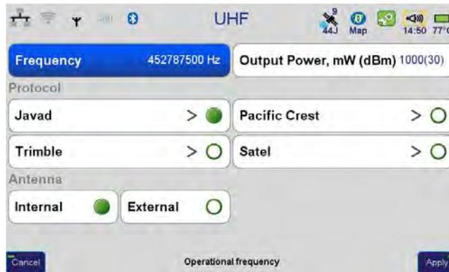
**Figure 3. UHF parameters**
