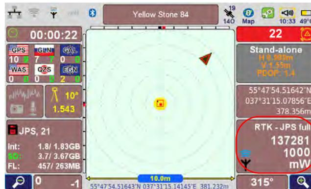
**Figure 20. Base station is transmitting corrections**
